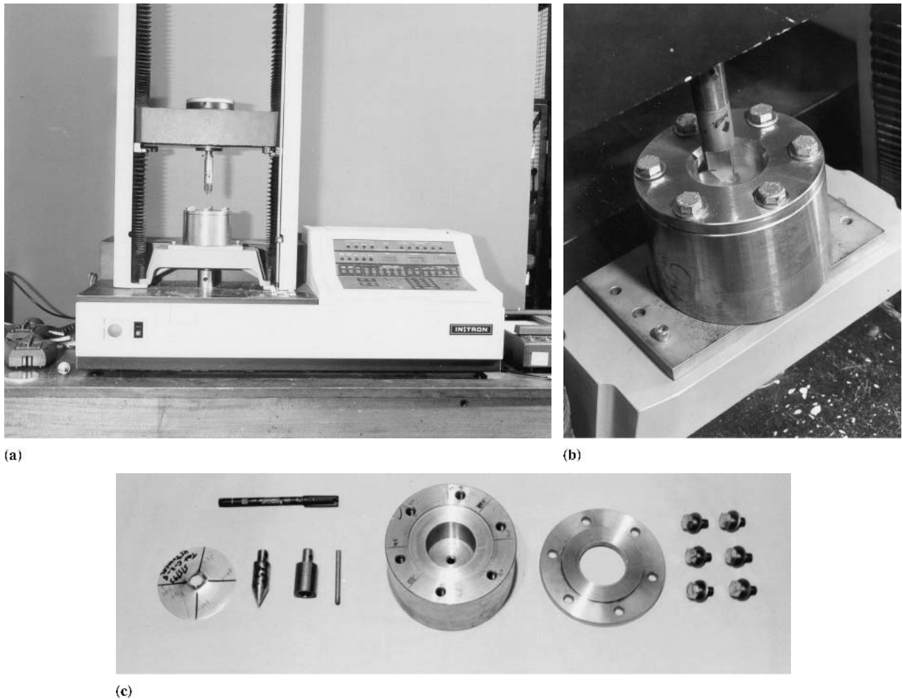
Fig. 1 Ball indentation experiment on Instron machine-specimen, die, cap, bolts, and ball assembly
